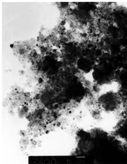
Fig. 7 Transmission Electron Micrograph (TEM) showing the decomposition product of a 2:0.5:0.5 mixture of \text{Fe}(\text{Ac})_2 , \text{Co}(\text{Ac})_2 and \text{Ni}(\text{Ac})_2 in the flow reactor at 300 °C and 25 MPa (run 12). Bar = 100 nm. The material looks very similar to those shown in Fig. 4a and 6.
